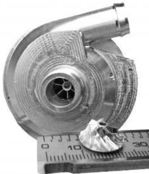
*Figure 3: Miniaturized turbo-compressor with gas bearing.*
