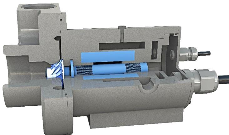
*Figure 1: Cross section of a gas-bearing turbo compressor.*
