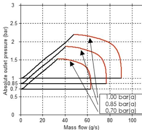
Fig. 6: Compressor map with absolute outlet pressure at constant inlet temperature (20°C)
