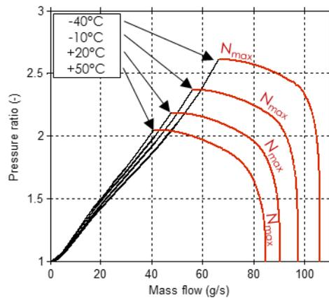
Fig. 7: Compressor map at constant inlet pressure (1 bar abs.)
