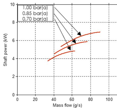
Fig. 5: Power map at constant inlet temperature (20°C)
