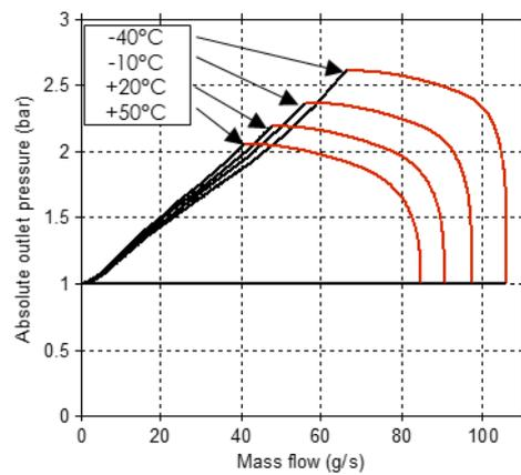
Fig. 9: Compressor map with absolute outlet pressure at constant inlet pressure (1 bar abs.)
