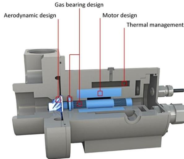
*Fig. 1: Sectional view of an air bearing turbo compressor*
