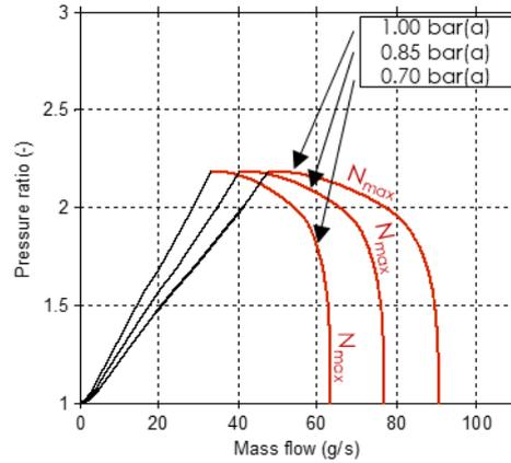
Fig. 4: Compressor map at constant inlet temperature (20°C)
