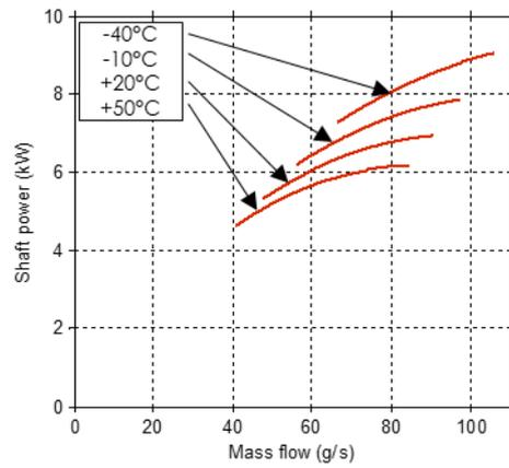
Fig. 8: Power map at constant inlet pressure (1 bar abs.)
